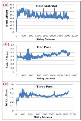
Fig: 12. Varation of friction coefficient Vs sliding distance in (a) Base Material (b) FSPed One Pass sample (c) FSPed Three pass sample
