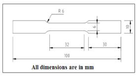
Fig: 2. The Tensile Test Specimen Dimensions
