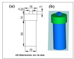
Fig: 1. (a) Dimensions of FSP Tool (b) Schematic diagram of the Tool
