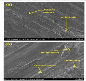
Fig: 13. SEM image of worn out surface of (a) Base Material (b) FSPed three pass specimen
