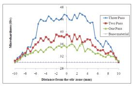
Fig: 4. Microhardness of the stir zone of the Processed Samples
