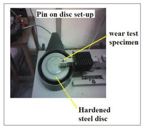
Fig: 8. Typical Pin on disc wear test set-up
