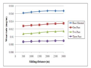
Fig: 10. Change in wear rate with Sliding Distance of Base Material and FSPed Samples
