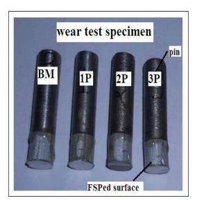
Fig: 9. Typical wear Test Specimens Extracted from the Processed Surface Layer
