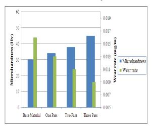
Fig: 11. Change in wear rate of base material and FSPed samples Vs Microhardness
